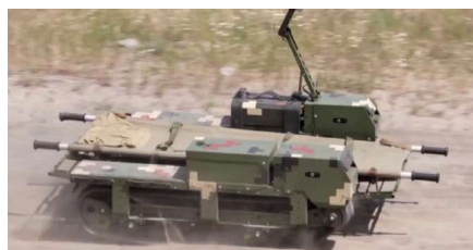
Figure 1 Example of an uncrewed ground vehicle (UGV) piloted by fibre-optic cable used for casualty evacuation.
