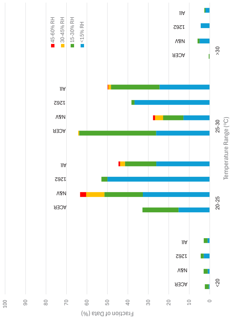
FIGURE 5-2 Distribution of in-flight temperature and humidity data from three independent datasets (Nicholls and Vink, ACER, ASHRAE 1262). NOTE: RH = relative humidity; N&V = Nicholls and Vink; 1262 = ASHRAE 1262. SOURCES: Created with data from ACER (2025), ASHRAE (2026), and Nicholls and Vink (2025).
