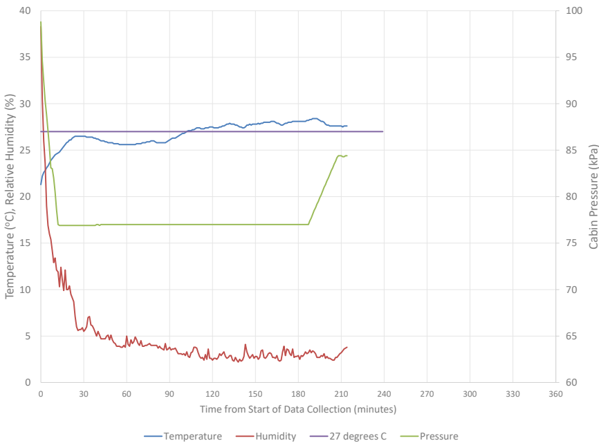
FIGURE B-12 Cabin environment conditions for Flight F031. NOTE: 27°C (80°F) represents the ANSI/ASHRAE Standard 161-2023 upper allowable limit for in-flight cabin temperature. SOURCE: Created with data from the ASHRAE-1262 data set (ASHRAE, 2026).
