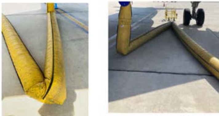
FIGURE 2-8 Examples of kinked hoses connecting preconditioned air units to aircraft.
